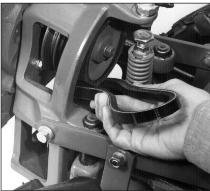
Figure 5-20: Shift into FORWARD and remove the belt.
